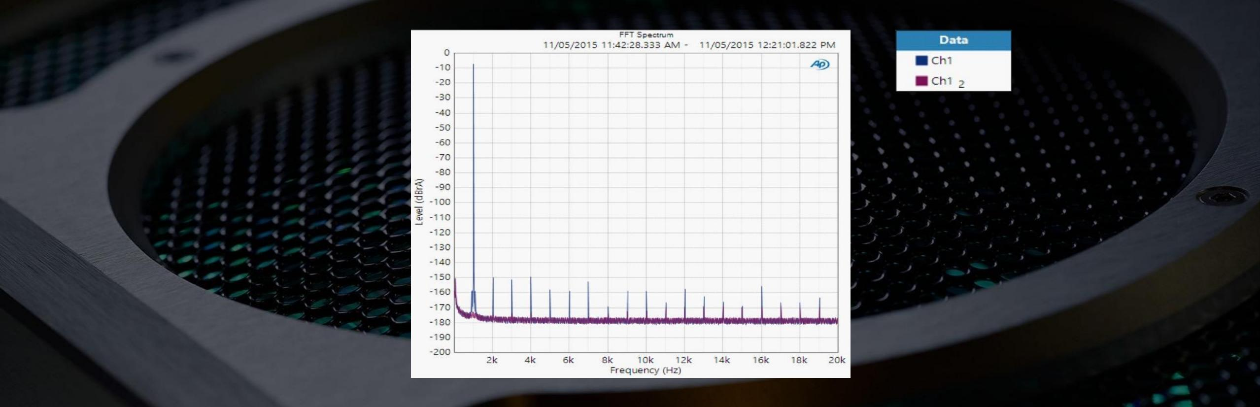
Blue 2.5v RMS, red no signal zero noise floor modulation. Noise floor at -178 dBA, distortion peaks -150 dBA, no anharmonic distortion.
