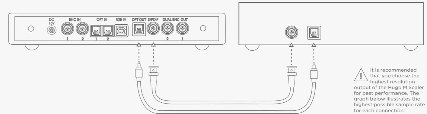
It is recommended that you choose the highest resolution output of the Hugo M Scaler for best performance. The graph below illustrates the highest possible sample rate for each connection:
