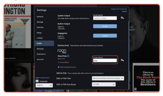
Choose Poly as the active zone by clicking on the radio button to the left side of Poly. Your Poly is now set up for use with Roon. Click anywhere outside of the Zones window to close it.
