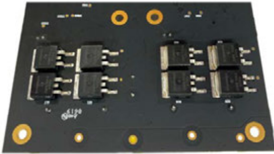
Output Devices: 8 x 1000 MOSFETs/Channel
